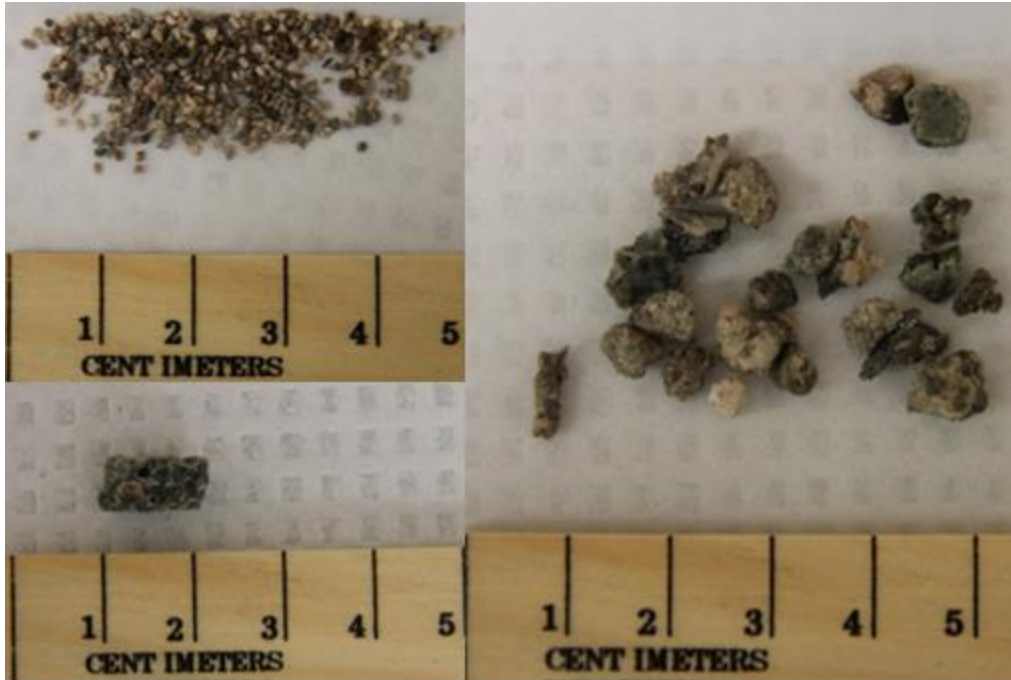
Figure 21. Examples of fallout particles prior to mounting and polishing.
