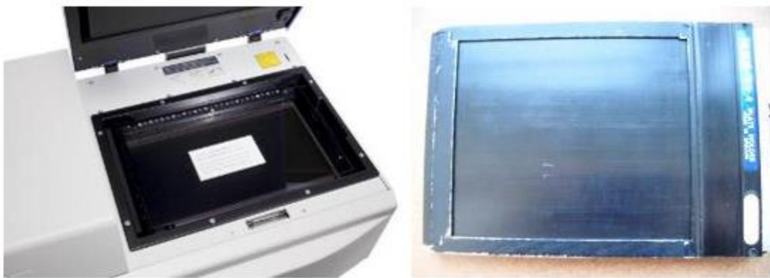
Figure 24. Typhoon scanner and standard film cassette used for the autoradiography.
